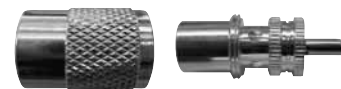
Male Solder Type 2 Piece Construction 401DTS PL-259 for RG-8, 213 Cable, Teflon Insulated, Silver Plated Body & Nut, Gold Plated Pin, Machined Brass
